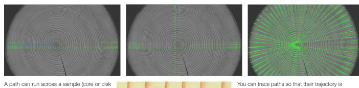
A path can run across a sample (core or disk radius) on a straight line. Hundreds of paths can be created with a single mouse click in predefined directions around the clicked position. Paths can aslo be created by clicking at their beginning and ending points.
