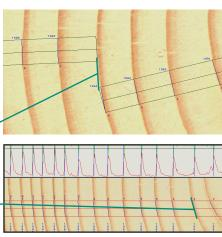
You can trace paths so that their trajectory is perpendicular to ring boundaries (as in manual dendrochronological measurement methods).
